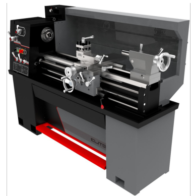
FULL LENGTH ENCLOSED SPLASHGUARD CONTAINS CHIPS AND COOLANT
