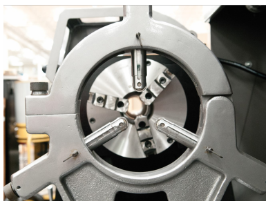
STEADY REST FEATURES DOUBLE SEALED BALL BEARING GUIDES FOR SMOOTH MATERIAL MOVEMENTS
