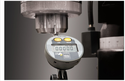
INDUSTRY LEADING SPINDLE TAPER RUNOUT OF 0.00012" ENSURES STRICT TOLERANCES
